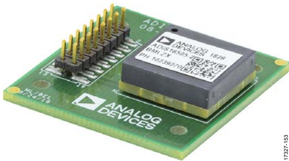
Figure 56. ADIS16500 Breakout Board (ADIS16505-2 Shown)
